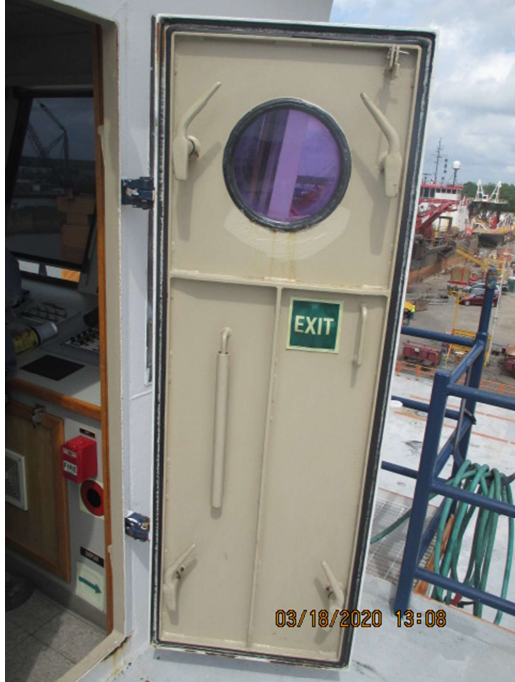
Weathertight door on Stbd bridge wing
