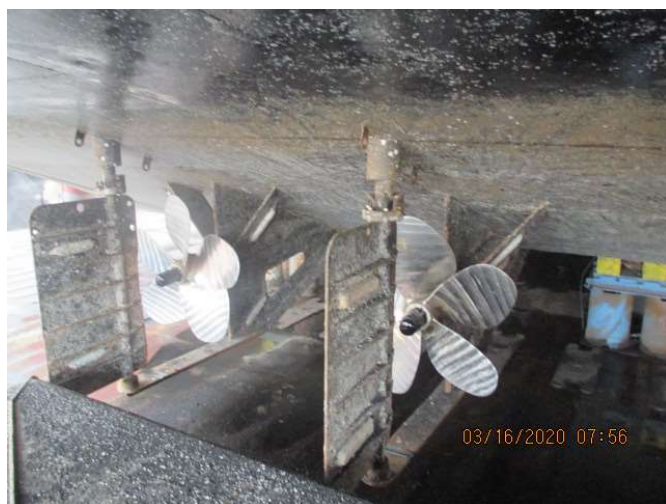
Port side outboard and inboard propeller
