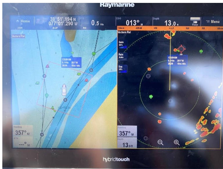
Figure 5. Display from Vessel RX at range rings of 1/8 NM. The location of Vessel TX is shown on the radar display as target "CG29109".
