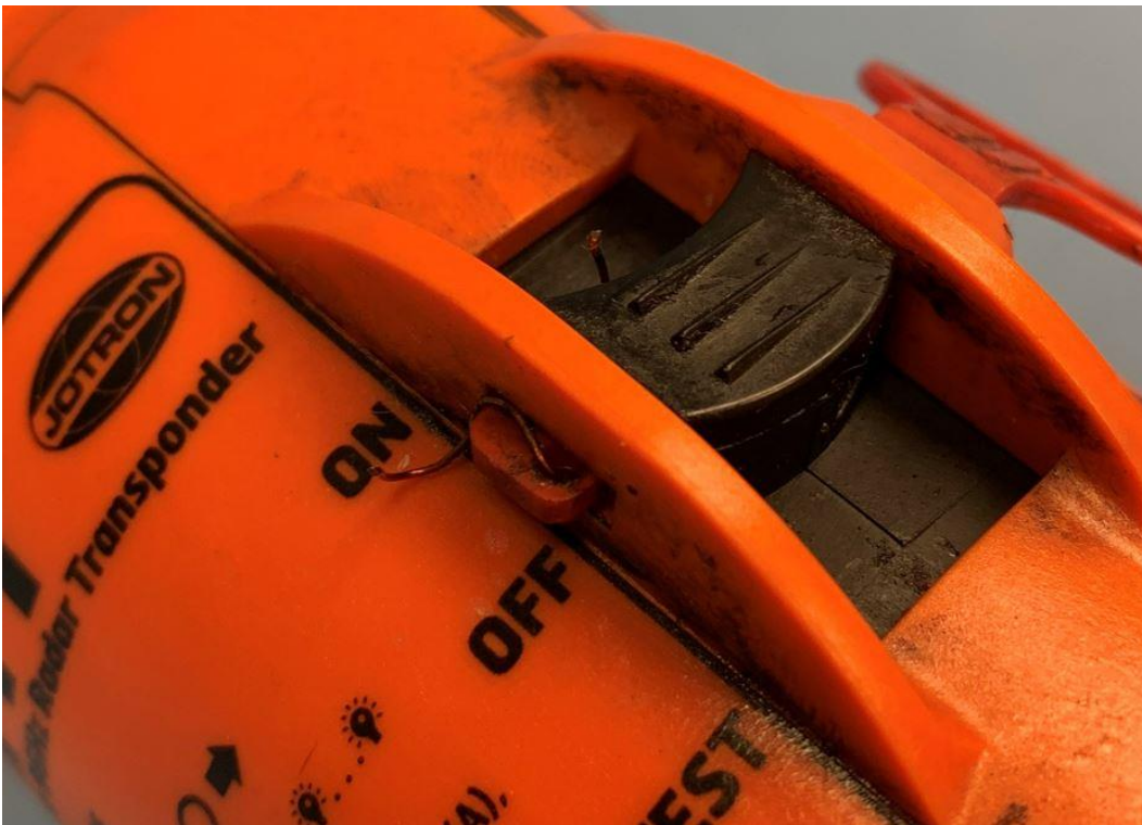
Figure 2. Broken safety wire (copper color) indicating the device had been activated at some time.
