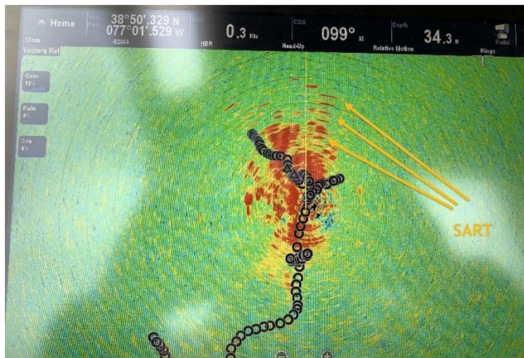
Figure 14. A picture of the radar display of the USCG vessel's radar display detecting the SART at a range greater than 0.4 NM and with the gain setting adjusted to 92%. The SART return has been annotated in yellow.
