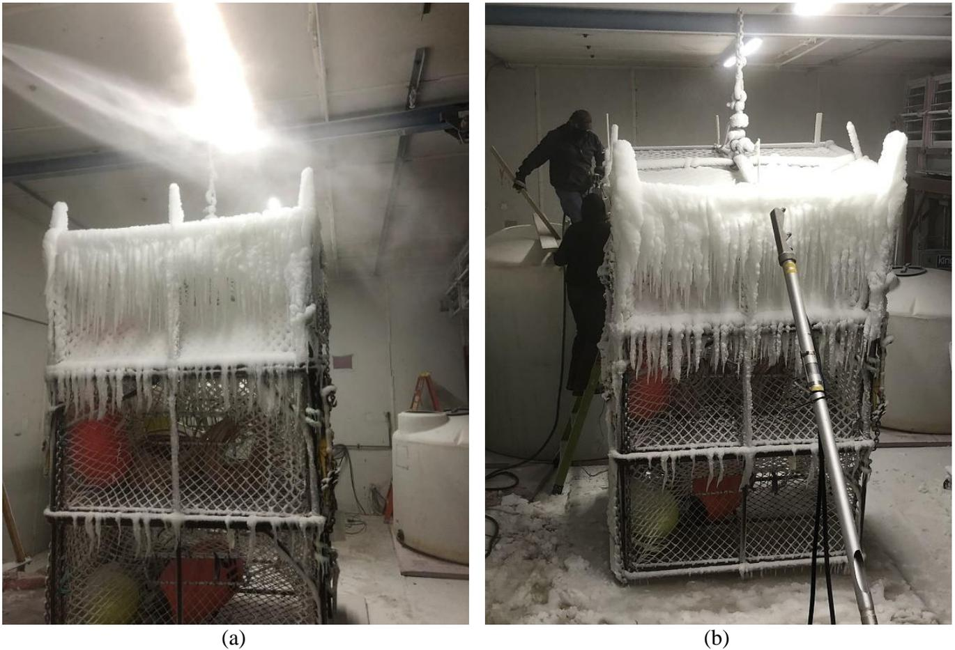
Figure 33. Test 8: (a) Accretion after approximately one hour spraying; face of top pot almost completely obscured, rules accreting ice well above frame top bar. (b) After 2-1/2 hours spraying, minimal accretion on far, top frame bar.
