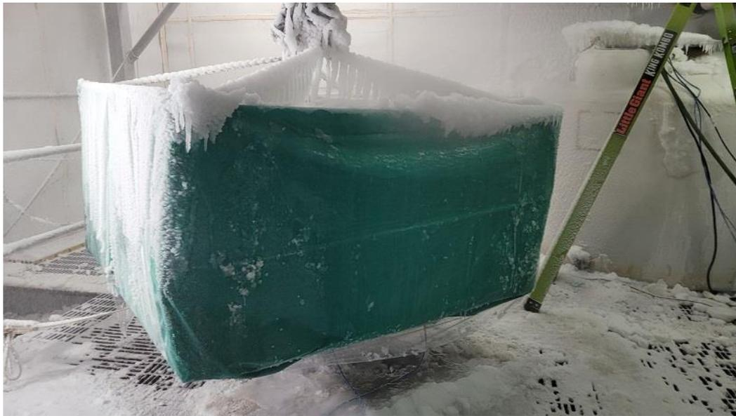
Figure 31. Test 7: Tarped crab pot, minimal to no ice accretion on side faces, but ice accretion on chain bridle and lip of tarp at top frame bar.
