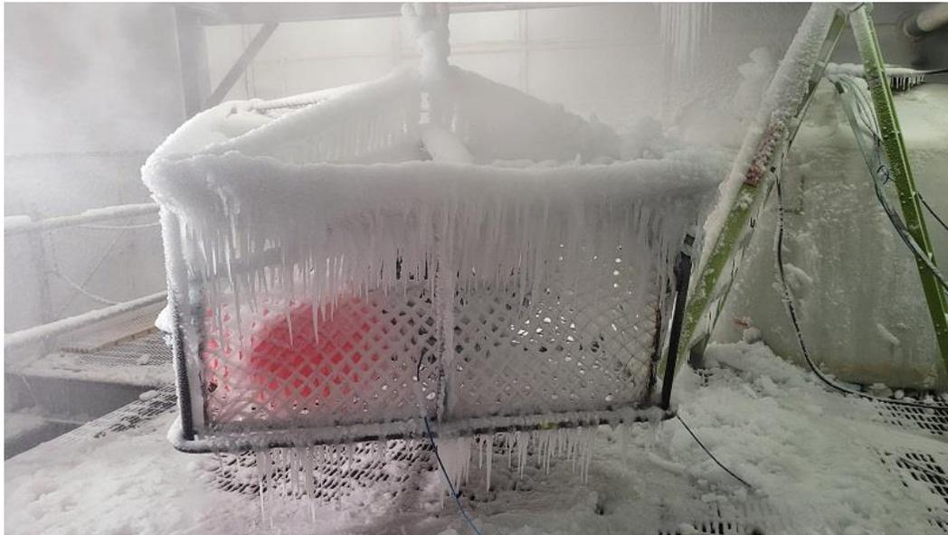
Figure 27. Test 5: Heavy ice accretion on top frame, mesh, and chain bridle, but very little inside.
