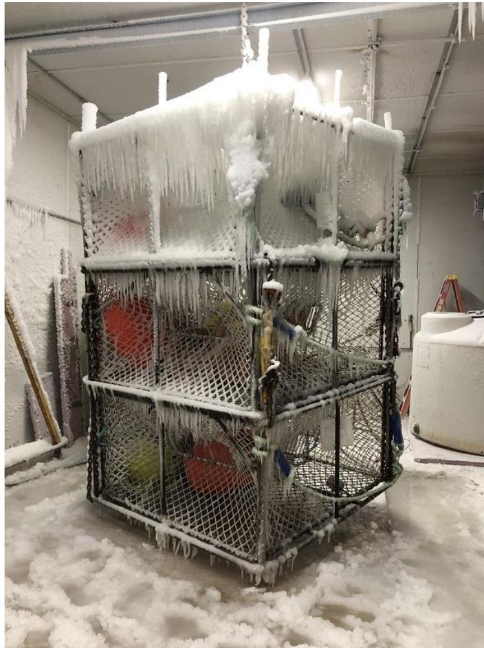
Figure 37. Test 10: Three-pot stack at the end of spraying.
