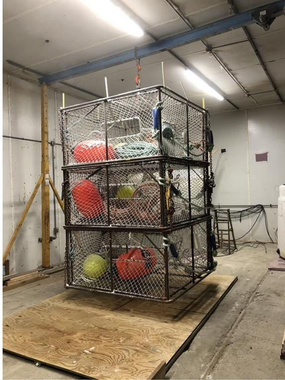
Figure 18. Three-pot stack in MEF suspended from load cell before test, with plywood ice removal “pan” underneath.
