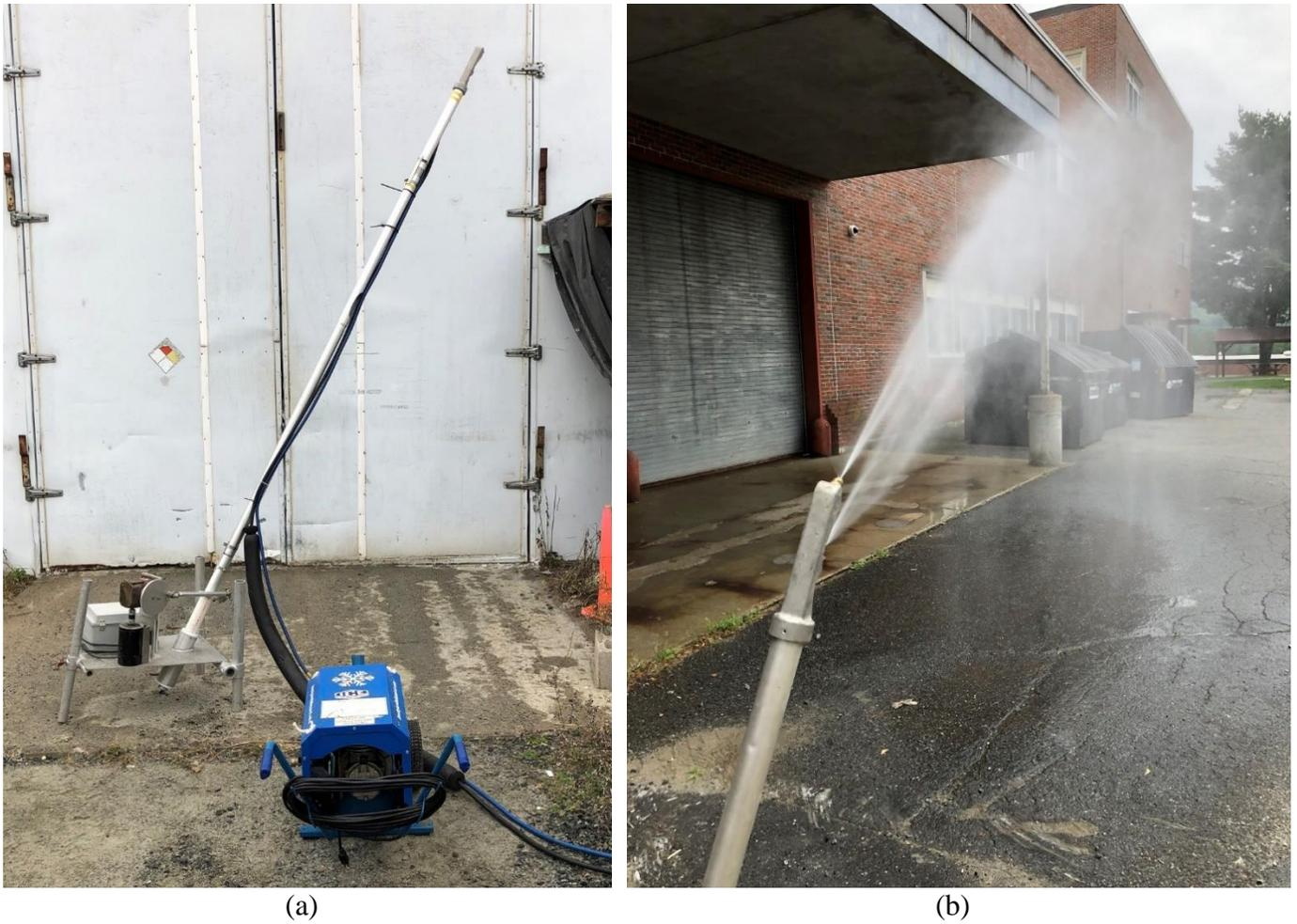
Figure 6. (a) Snowmaker with wand attachment and (b) close-up of spray pattern.
