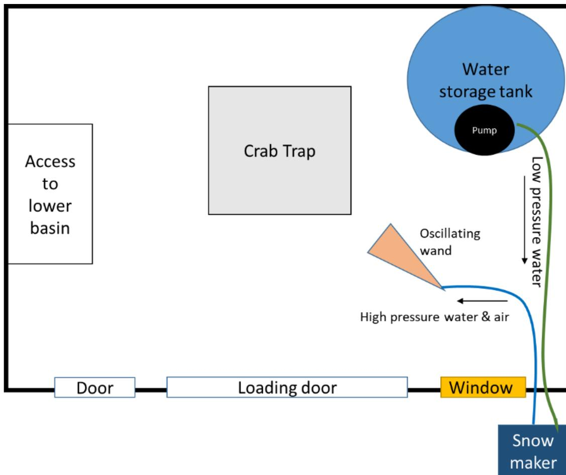
Figure 8. Schematic layout of the Cold-Pit for testing.
