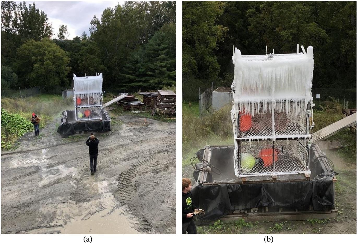
Figure 34. Test 8: Three-pot stack, outside after spraying (a) normal perspective at 45 ft distance (b) zoom perspective from 45 ft.
