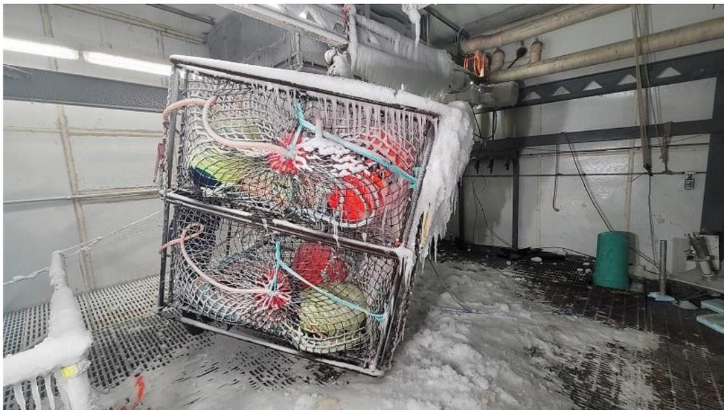
Figure 30. Test 6: Side of two-pot stack showing minimal accretion on mesh, both pots.
