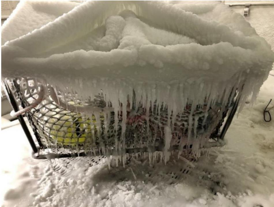
Figure 22. Test 1: Heavy accretion on top frame, mesh, and bridle.
