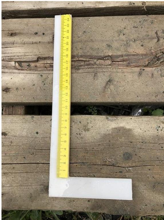
Figure 19. Delrin® measurement rule used in three-pot stack testing.
