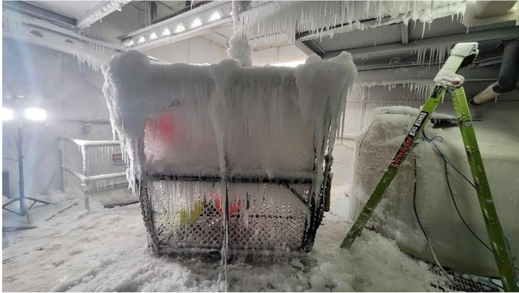
Figure 29. Test 6: Two-pot vertical stack showing heavy ice accretion on spray-facing side with iced-over mesh, large buildups on corners and top bar, and numerous icicles.
