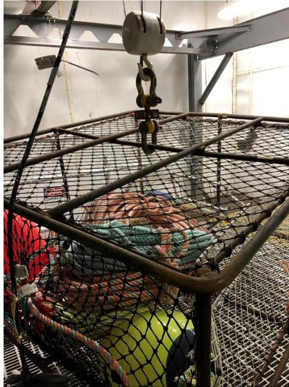
Figure 9. Single pot suspended from load cell prior to trial experiment.
