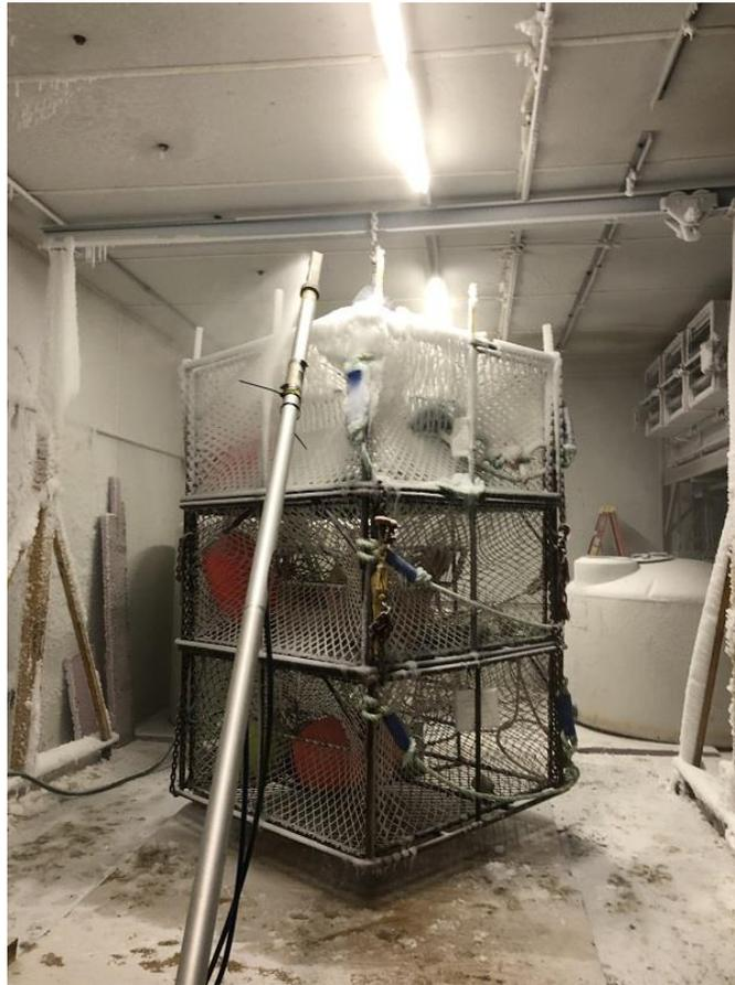
Figure 36. Test 10: Ice accretion on the top pot of the stack after adjusting sprayer location.
