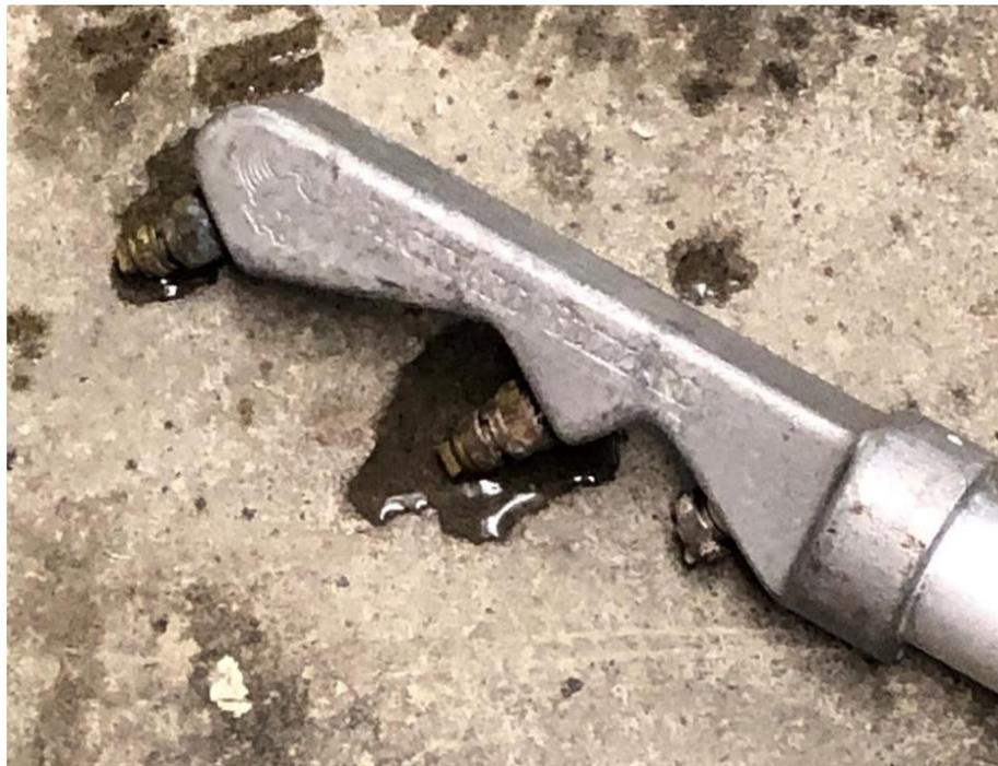
Figure 11. Snow-maker spray wand nozzle head thawing after 20 minutes of use.
