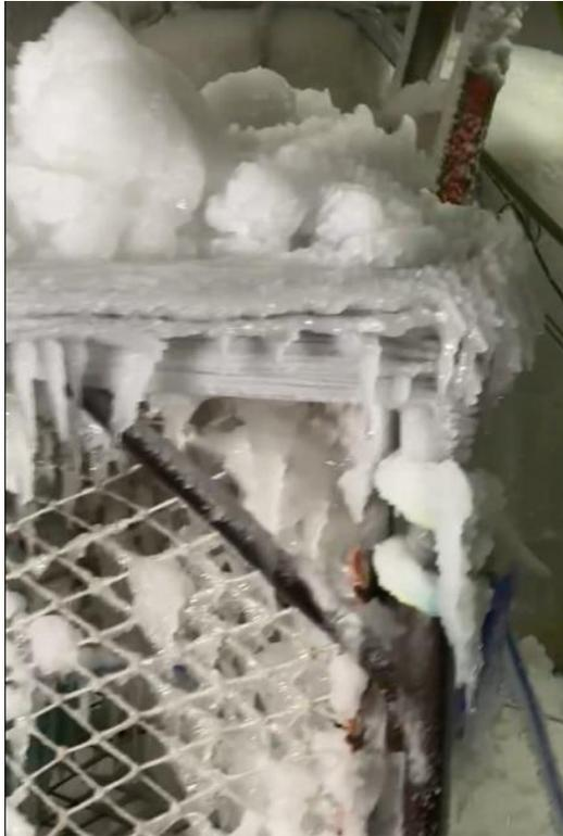
Figure 28. Test 5: Top frame bar (closest to camera) wrapped in plastic, showing minimal accretion after 30 minutes spraying as compared to chain bridle (top right of image).
