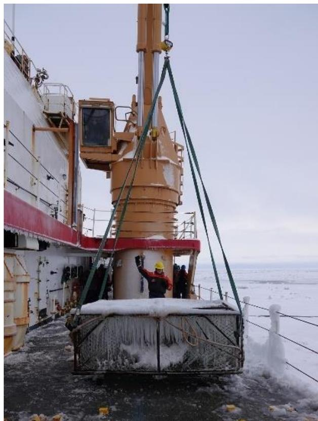
Figure 3. Hoisting crab pot to weigh after accretion.
