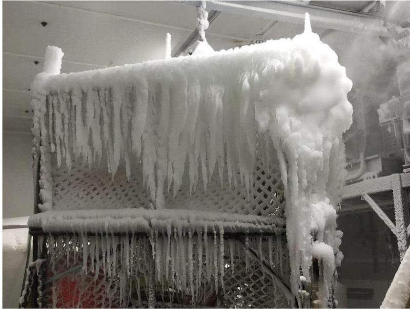
Figure 39. Test 11: Large ice accumulation extending 10-12 inches from the spray-facing corner.
