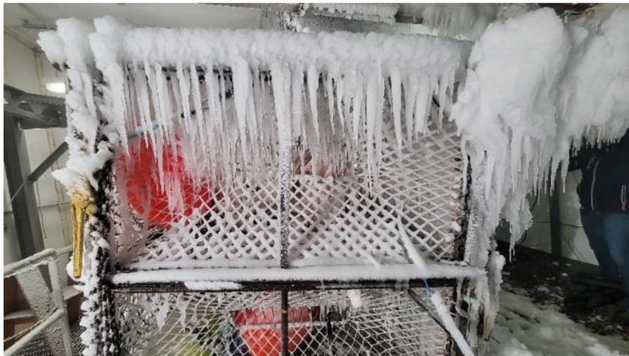
Figure 26. Test 4: Ice accumulation on top bar with large protrusion from the spray-facing corner.
