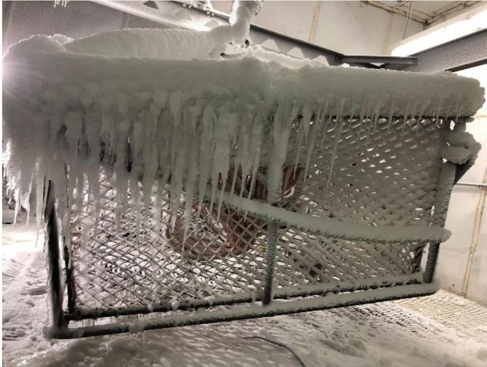
Figure 23. Test 2 ice accretion at end of spraying.
