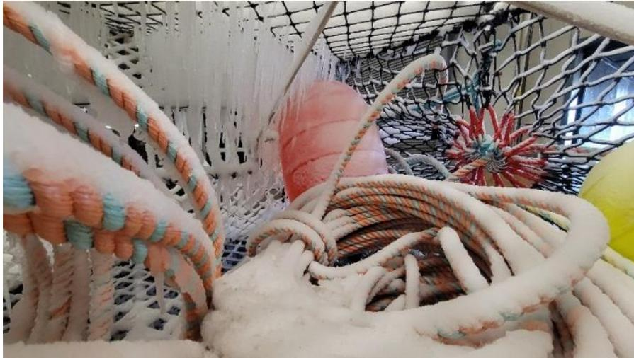
Figure 25. Test 4: Interior of top pot showing icicles and minimal accretion.
