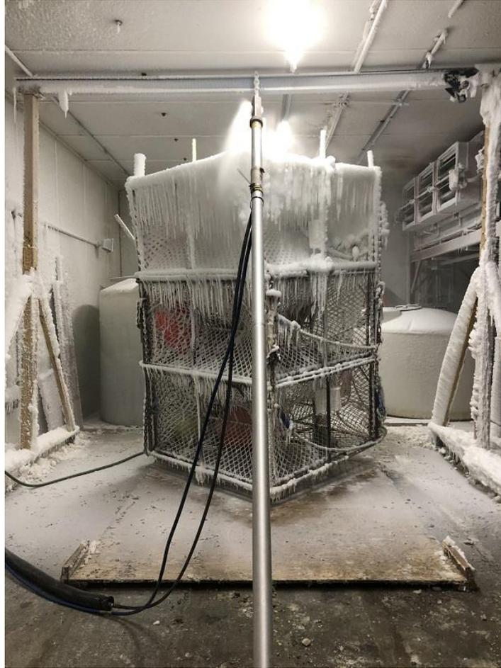
Figure 38. Test 11: Thirty minutes into continuation of spraying adding to Test 10 accretion.
